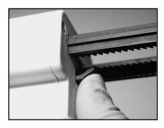
Flip up the cartridge lock and seat the cartridge in the gun. (The notch in the base of the cartridge should face downward as in the photo.)
