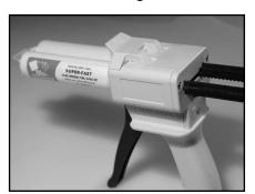
4. Before affixing the mixing tip: Remove the cap that seals the cartridge by twisting the cap counterclockwise and pulling it from the cartridge. Discard the cap.
